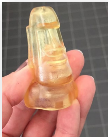
3D-printed biobased resin developed at PL12
